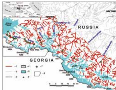
Fig. 1 - Map of debris flow channels for study area. Legend: 1 – river channels with traces of debris flows, 2 – rivers with no evidence of debris flows, 3 – boundary of Main Caucasus Range (and state boundary), 4 – towns and settlements, 5 – glaciers, 6 – mountain summits, 7 – areas of temporary stay for large numbers of people (ski resorts, mountain-nering camps etc), 8 – area, shown on the figure 2 (see below) (Compiled by Kapitanov A.N., Chernomorets S.S. and Tutubalina O.V. on the base of Landsat ETM+ satellite imagery of 2000-2001, aerial imagery of 2004, topographic maps at scales of 1:25000 to 1:200000 (various years), as well as field data of Seinova I.B., Dokukin M.D. and Chernomorets S.S.)
